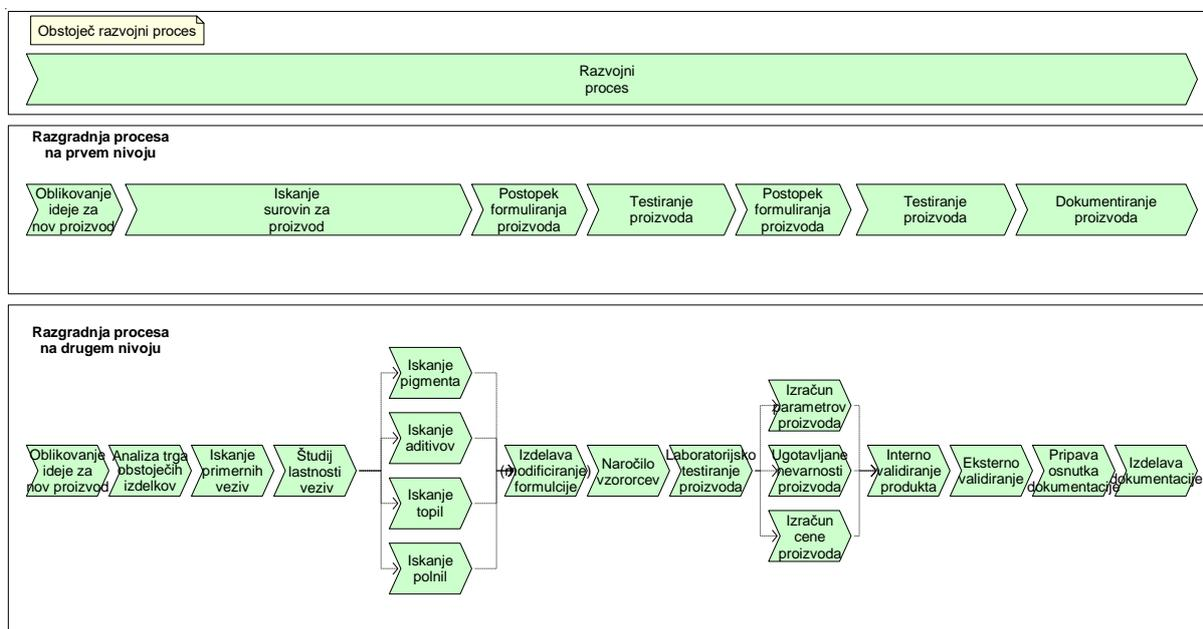
Figure 1: Example value added diagram of an existing development process for paints and coatings
