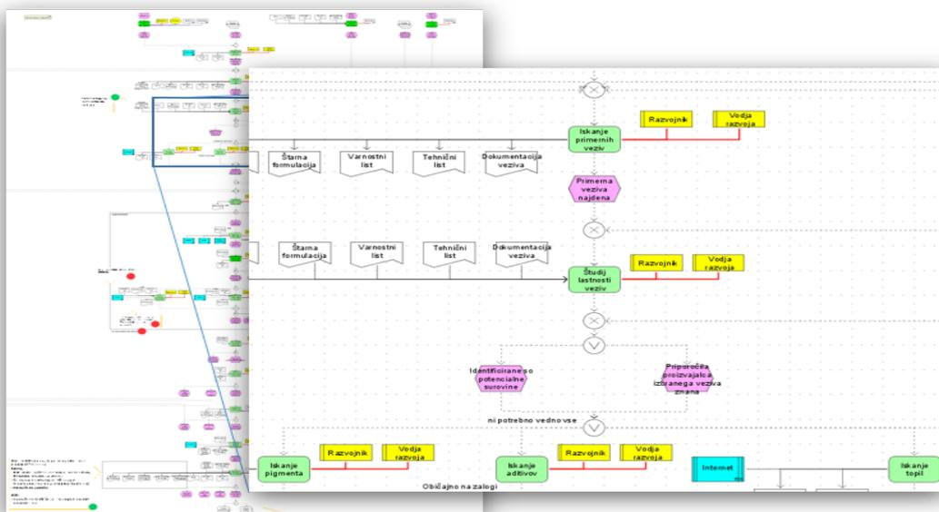
Figure 2: EPC model of existing development process for paints and coatings
